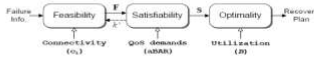
Fig. 3. Localized reconfiguration planning in ARS: ARS generates a reconfiguration plan by breaking down the planning process into three processes with different constraints.
